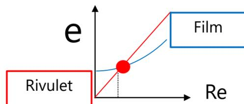
The principle of minimum energy gives the wet part of the solid surface
