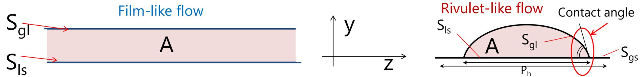
Energy of the flow = Kinetic energy + Surface tension energy
